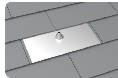
Step1: Put the flashing plate at the correct position
